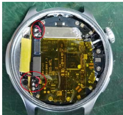
4. Screen with copper foil shielding
