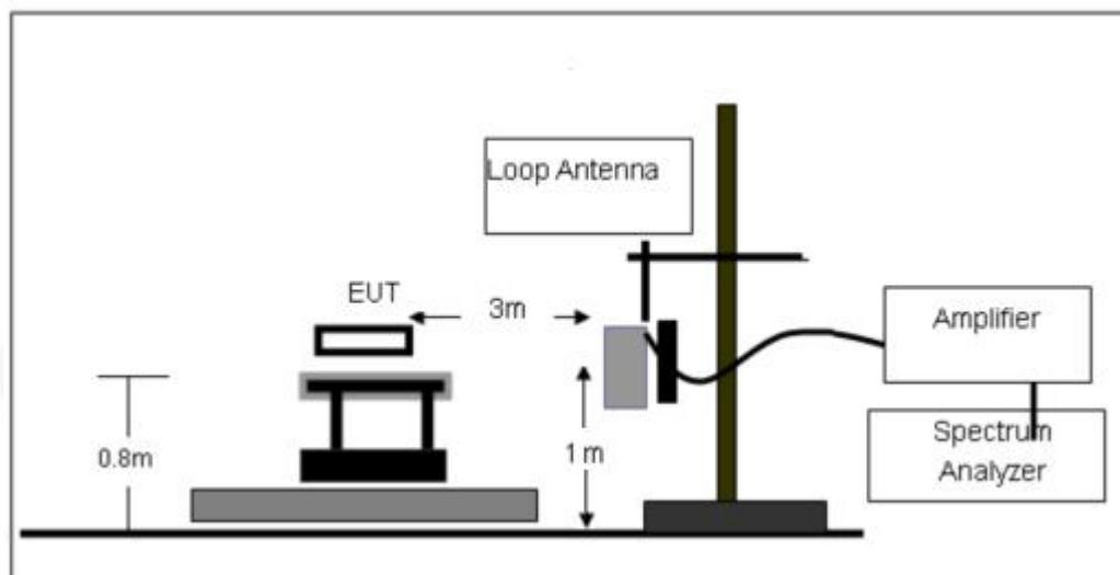
( B ) Radiated Emission Test-Up Frequency 30MHz~1GHz
