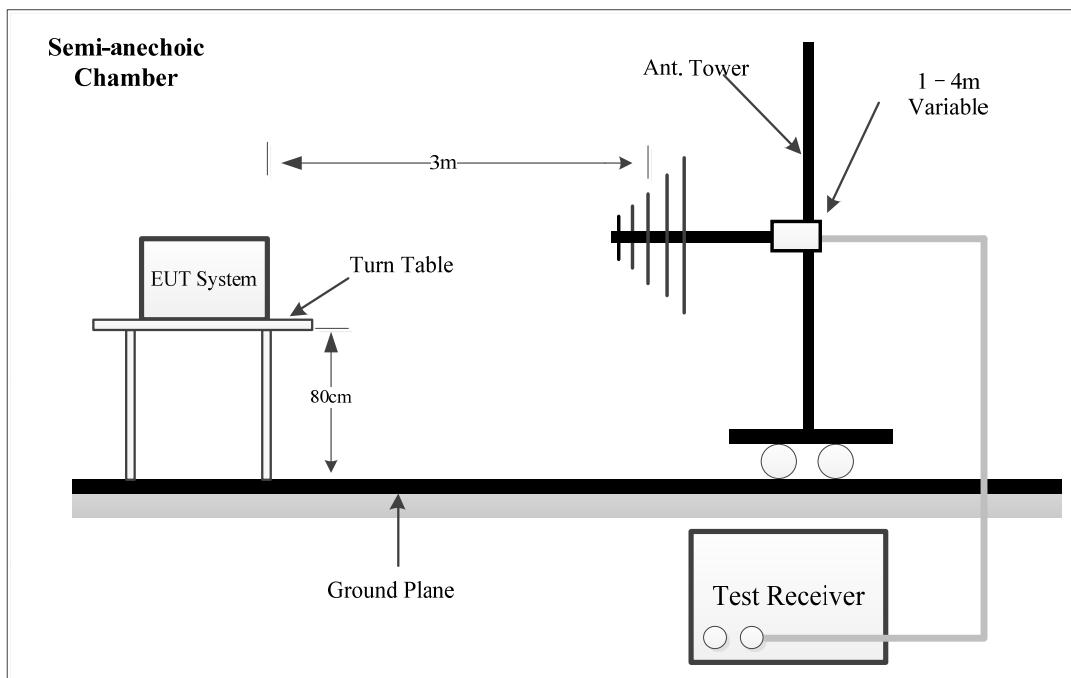
The radiated emission tests were performed in the 3-meter chamber test site, using the setup accordance with the ANSI C63.10-2013.
