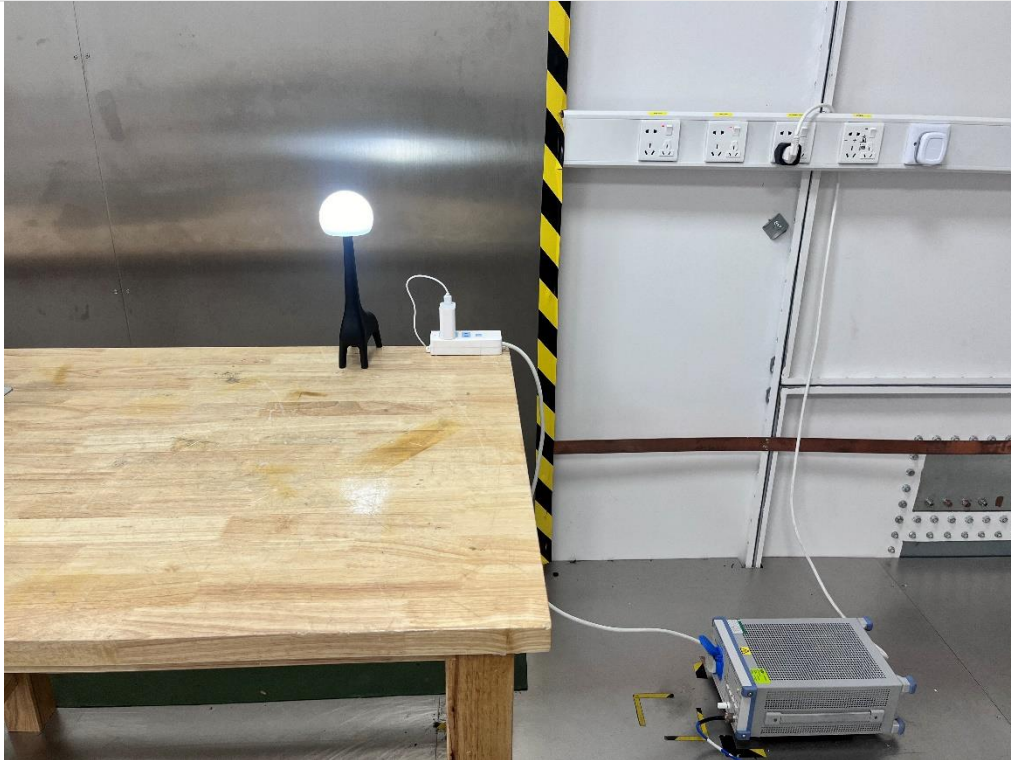
AC Power Line Conducted Emission
