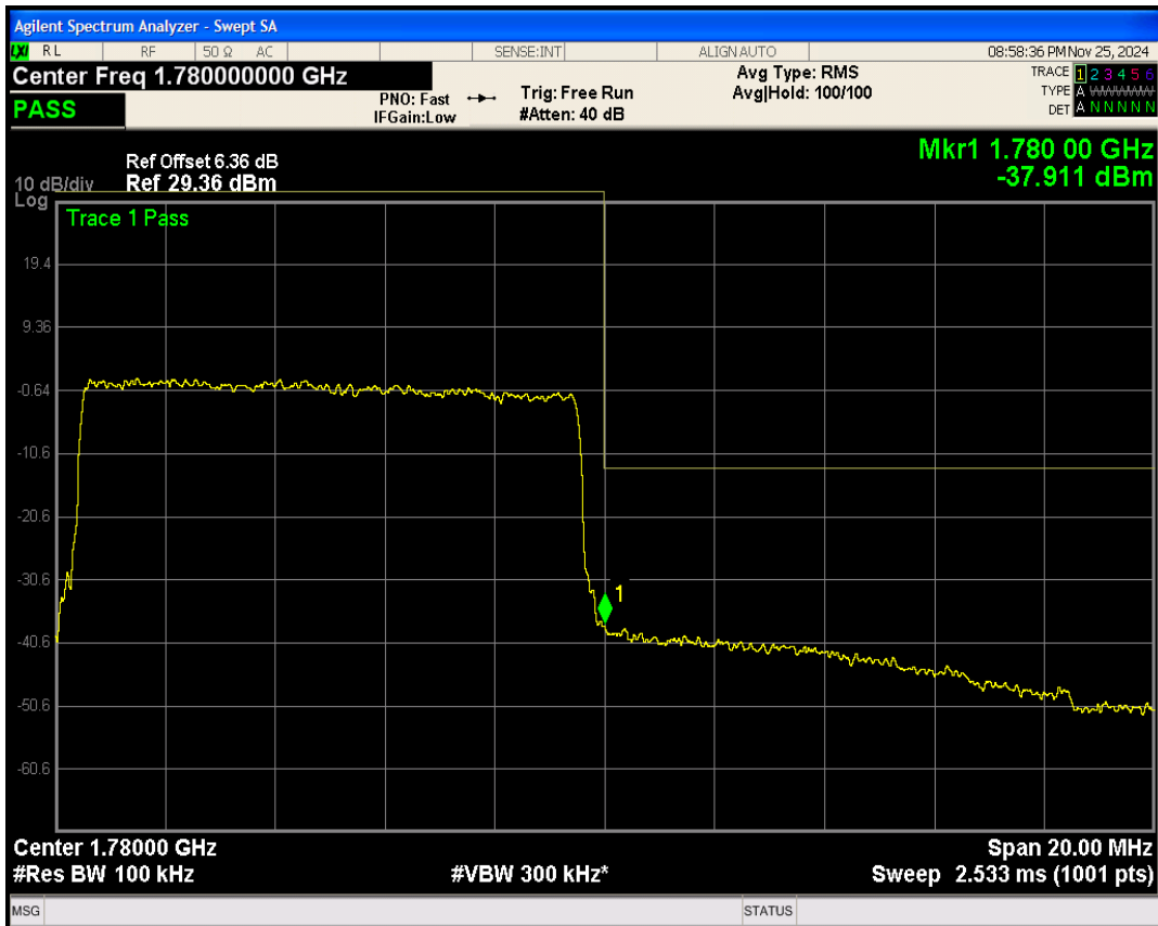
Band66 QPSK BW=15MHz Channel=132047 RB Size=75 Position=#0
