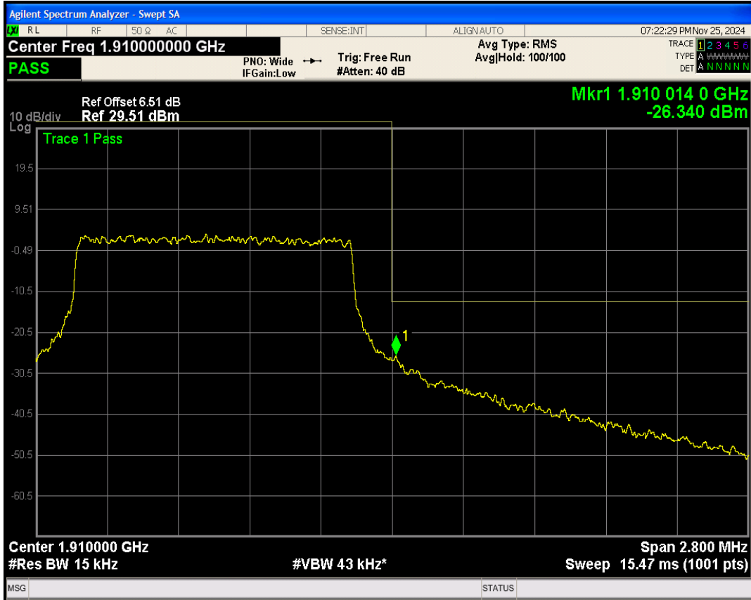
Band2 16QAM BW=3MHz Channel=19185 RB Size=15 Position=#0
