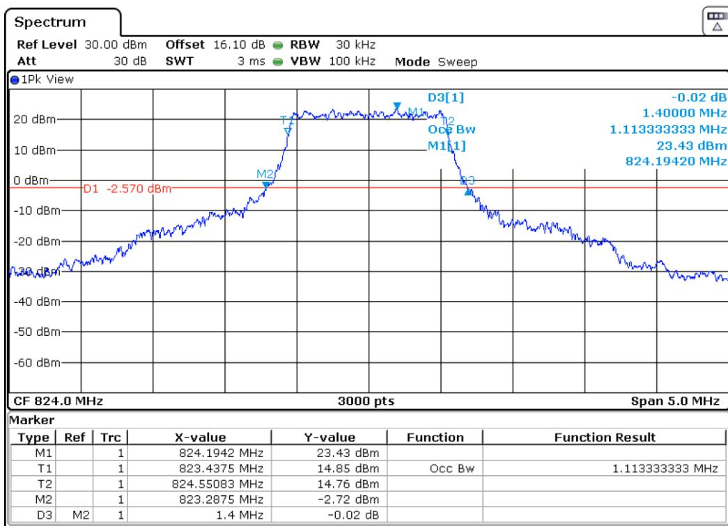
LTE 16QAM MODULATION. BW = 1.4 MHz
