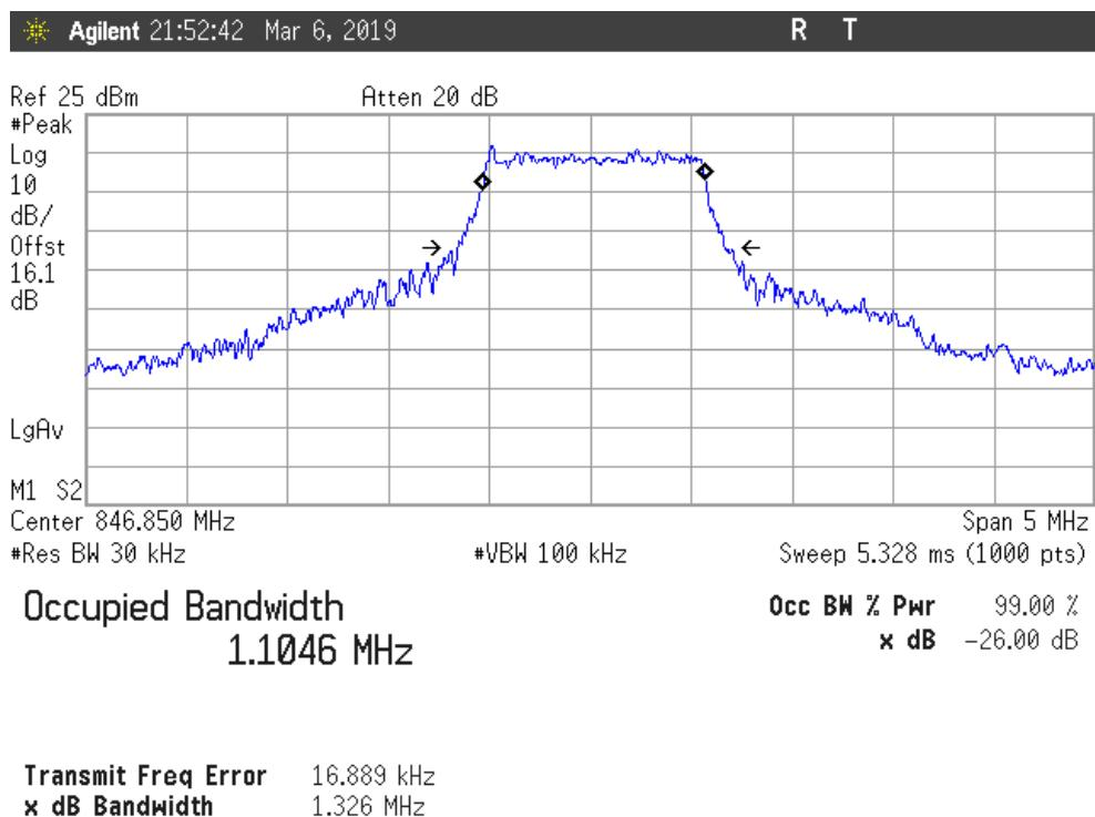
LTE 16QAM MODULATION. BW = 1.4 MHz (Band 5)
