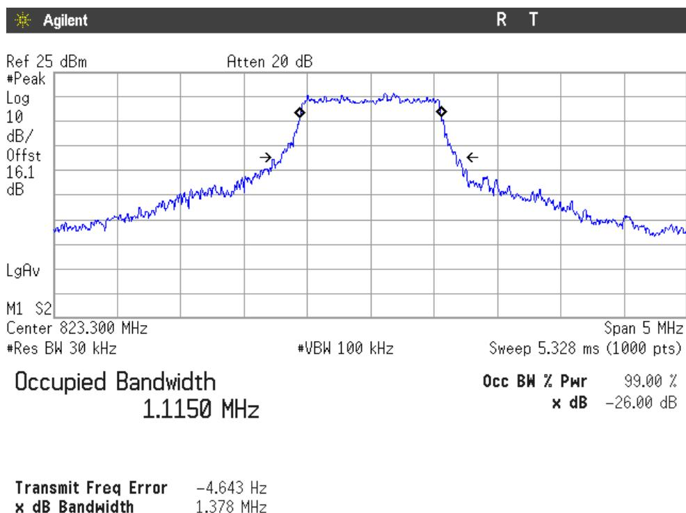
LTE 16QAM MODULATION. BW = 1.4 MHz (Band 26)
