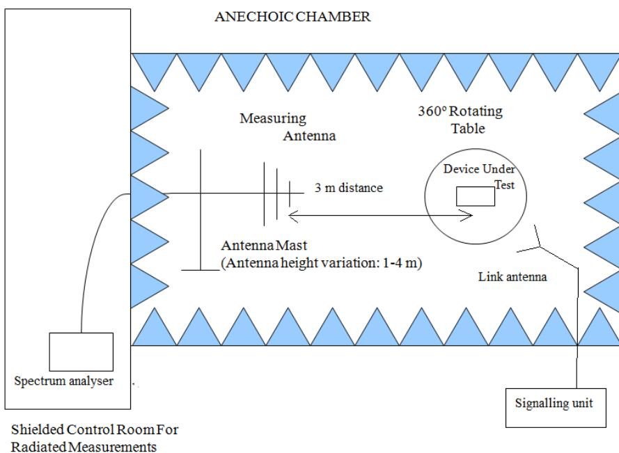
Radiated measurements above 1 GHz.
