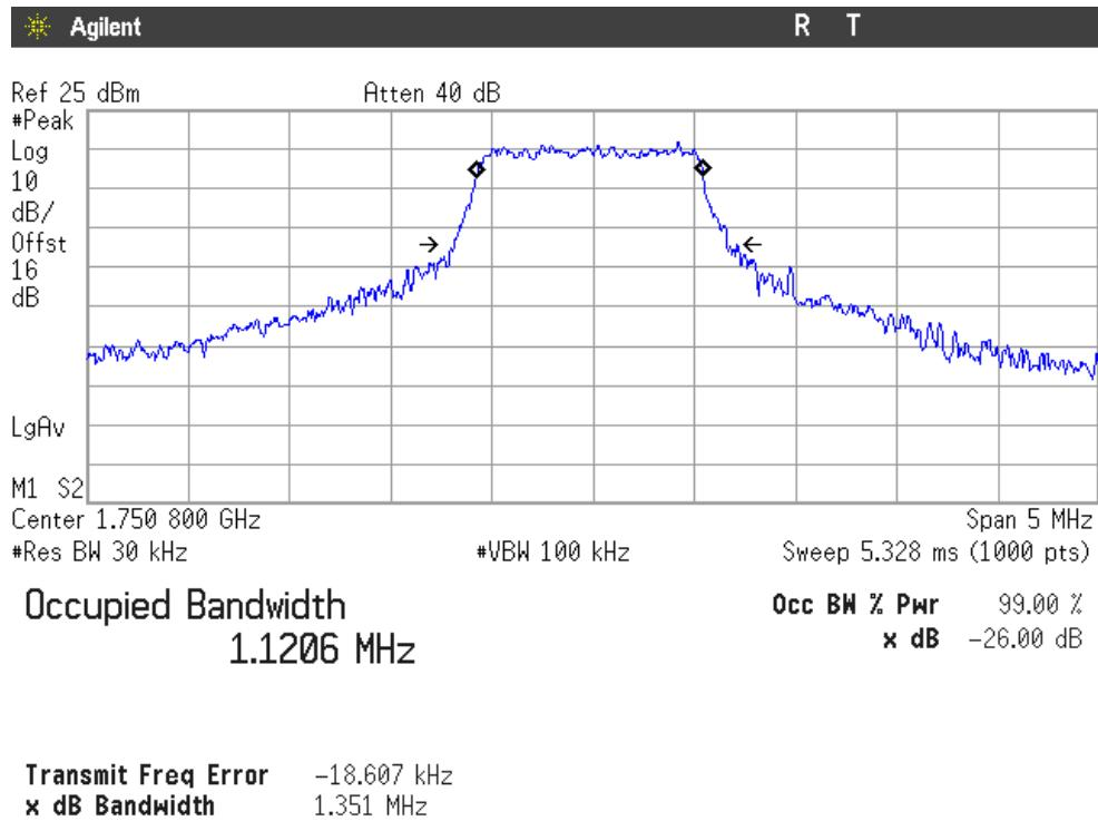
LTE 16QAM MODULATION. BW = 5 MHz (Band IV)
