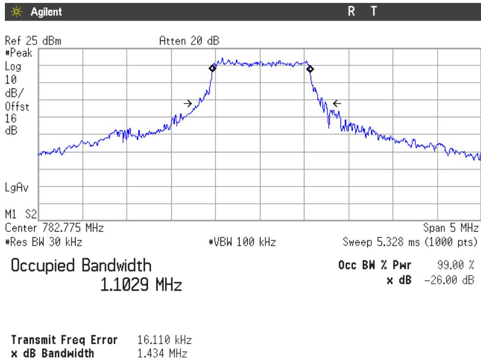
LTE 16QAM MODULATION. BW = 5 MHz (Band XIII)
