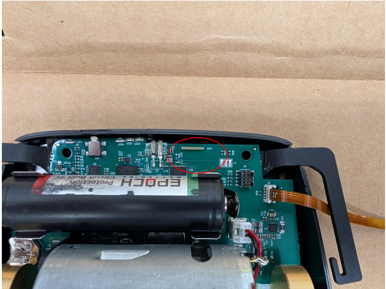
Close-up of the RF antenna layout in the MSP-09-2007 Vibration Pack
