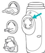
④Replace the national standard plug: press the button by the arrow shown in the diagram, and at the same time rotate counterclockwise to remove the plug to replace other plugs
