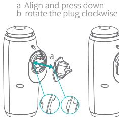
③Align the power plug bump with the device notch and press it tightly (such as A), rotate clockwise into the device, attach a foam pad under the plug, and select a suitable position to insert the socket
