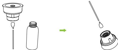
① Pull out the suction tube from the main body of the atomizer head and remove the original atomizer core.
