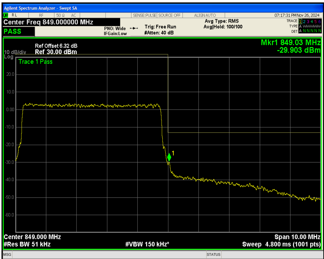
Band5 QAM16 BW=5MHz Channel=20625 RB Size=25 Position=#0
