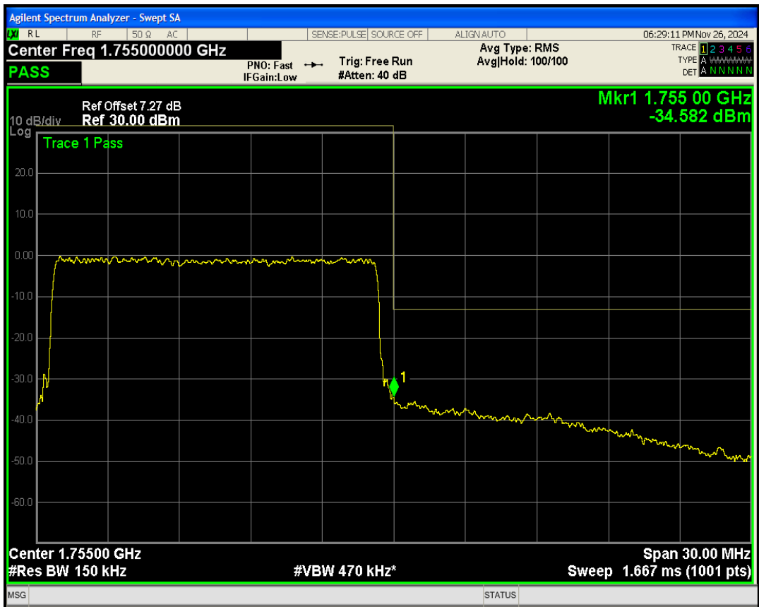
Band4 QPSK BW=20MHz Channel=20050 RB Size=100 Position=#0
