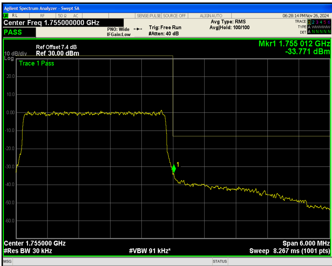
Band4 QAM16 BW=3MHz Channel=20385 RB Size=15 Position=#0
