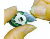
Remove the original battery and install a new battery
