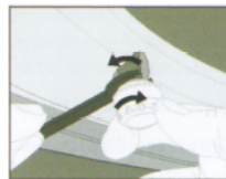
d. Tighten the sensor and tighten the anti-theft nut counterclockwise with a wrench
