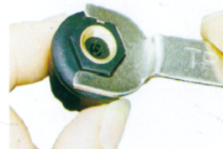
Open the outer cover with a wrench
