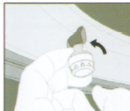
c. Screw the anti-theft nut counterclockwise against the sensor
