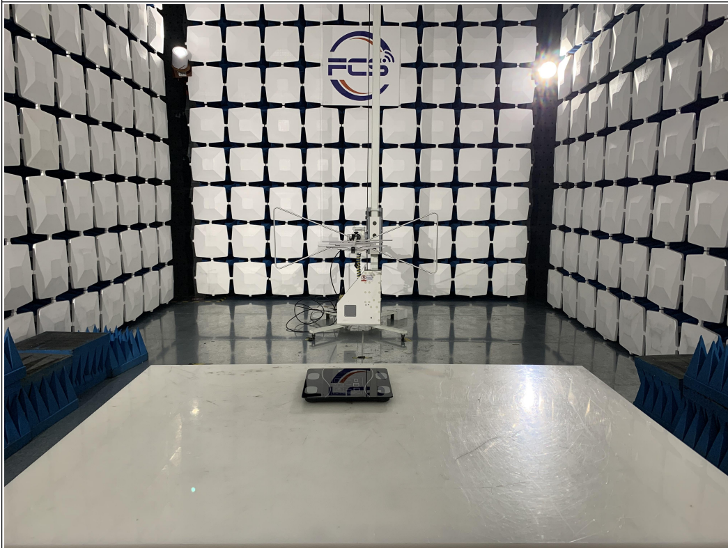
Above 1GHz for radiated emission test setup
