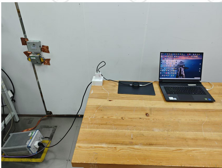
Conducted Emissions Test Setup
