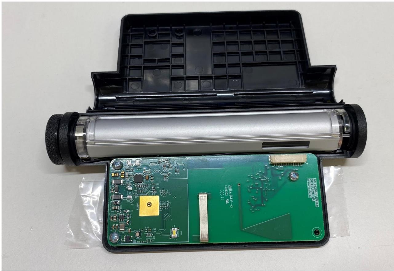
The PCB is screwed down onto the enclosure, and the silver tube is the battery tube for power.
