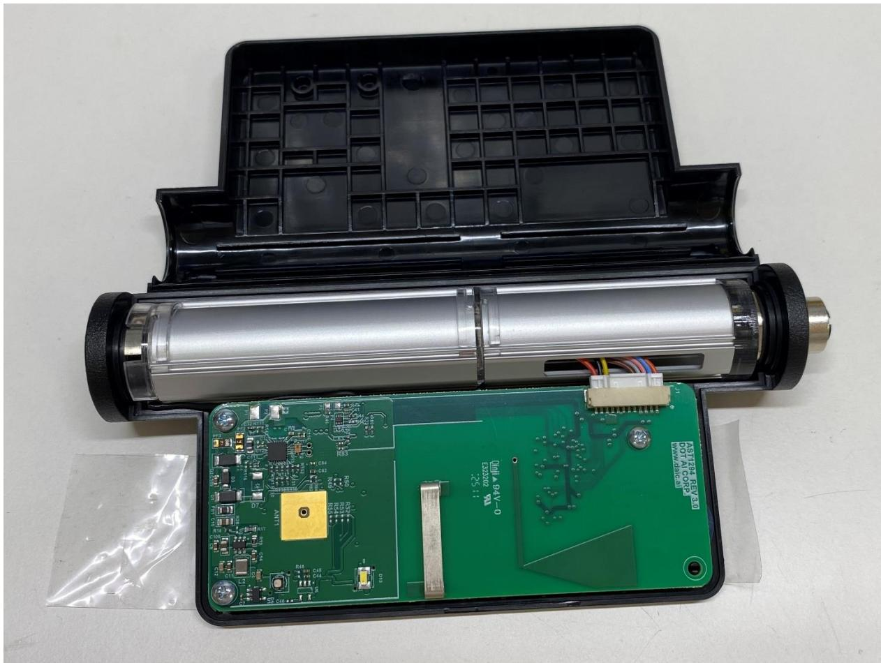
The PCB is screwed down onto the enclosure, and a J1 cable connects the M12 port and J1 connector on the PCB for power.
