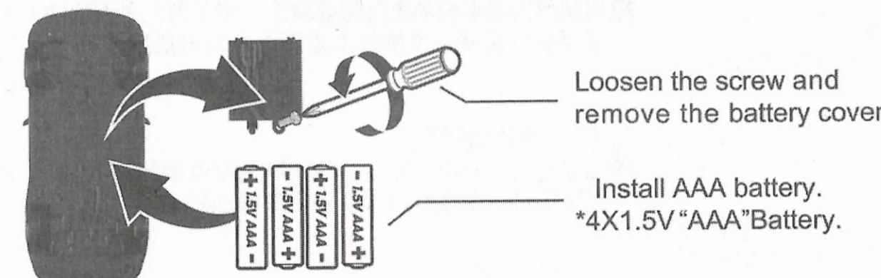
Loosen the screw and remove the battery cover.
