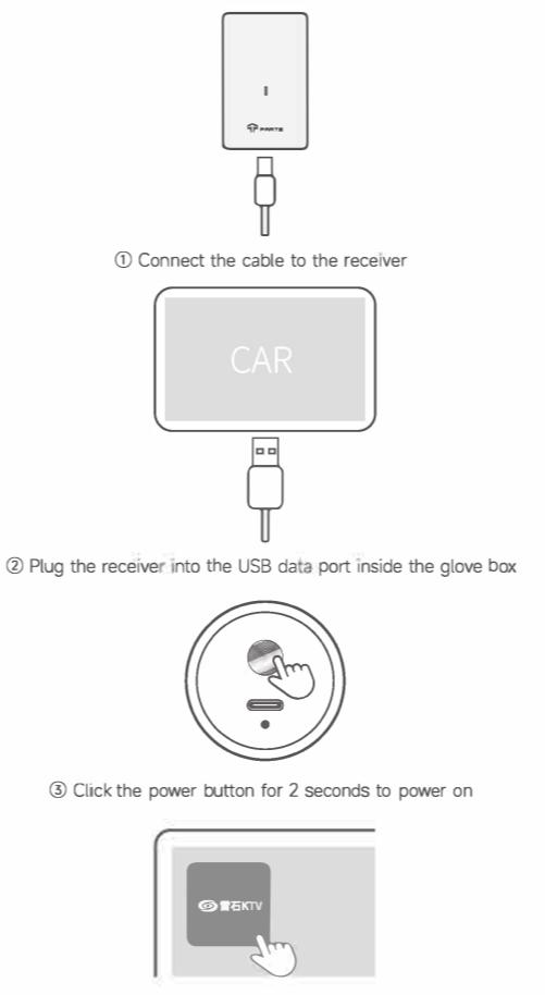
Note: Receiver should not be placed near large metal objects, and ideally there should be no obstruction between the microphone and receiver.
