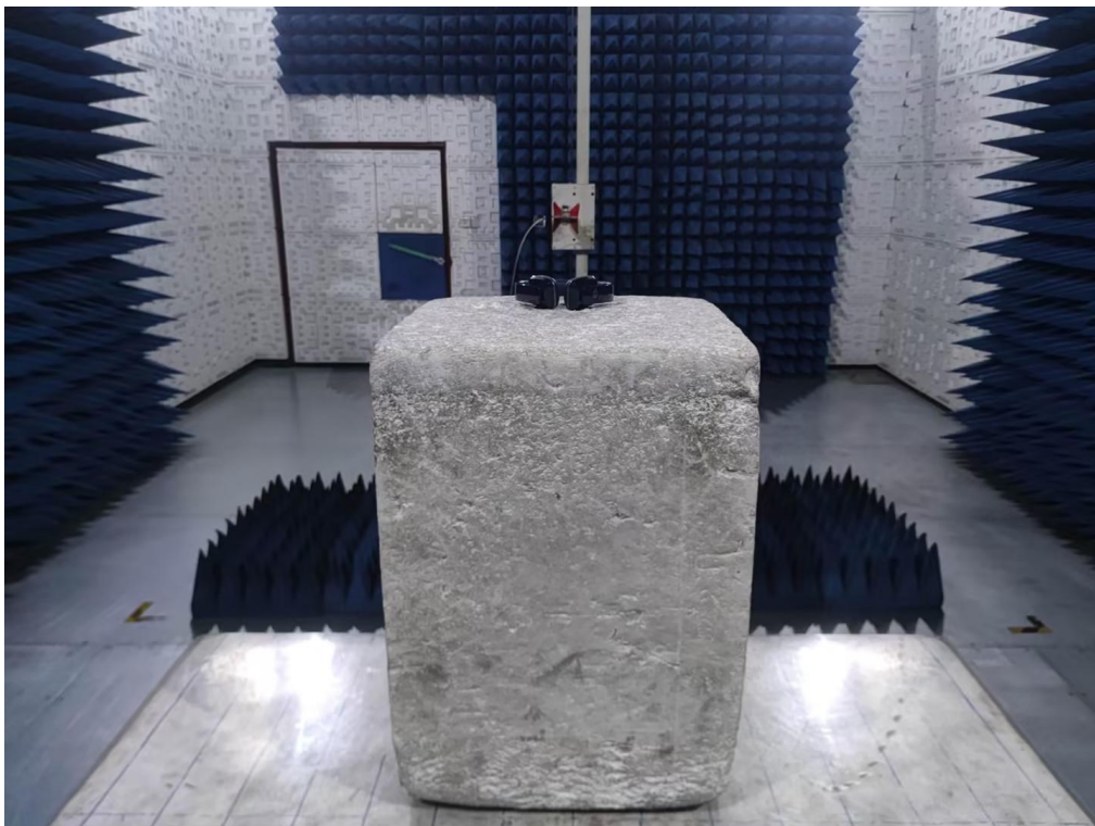
RADIATED EMISSION TEST SETUP ABOVE 1GHz
