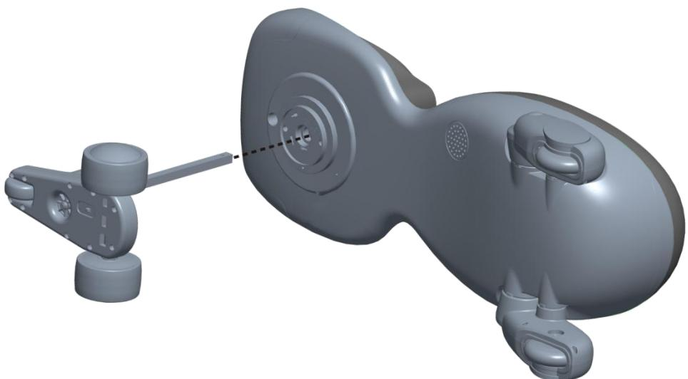
Please place the drive device with the square tube in the direction shown in the picture, pass the square tube through the round hole at the bottom of the car, and then lay the car flat on the ground.
