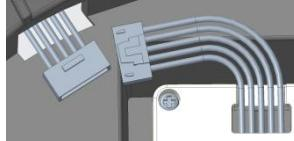
III Connect the two interfaces face up and check that the connection is tight
