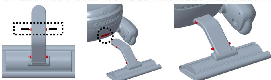
Press the square button on the mop handle in with your hand, insert the mop handle all the way into the bottom of the square slot under the vehicle body, then release the square button to secure the mop to the vehicle body. Please ensure it is firmly fixed before use. If you want to detach the mop from the vehicle body, press and hold the square button and pull the mop outwards.
