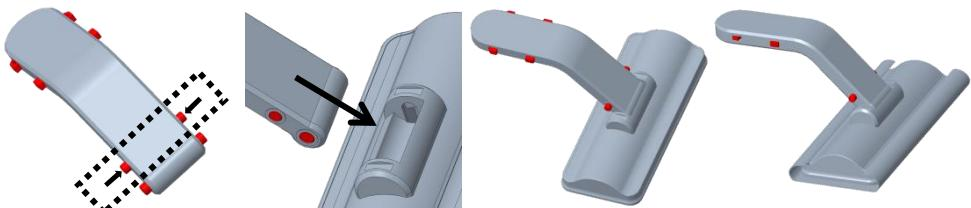
Press the cylindrical button on the mop handle in with your hand, insert the mop into the circular slot of the mop head, then release the cylindrical button to secure the mop handle and the mop head. Please ensure they are firmly fixed before use. Lay the disposable mop cloth under the mop head, and press the excess part onto the hook-type hook-and-loop fastener attached to the top of the mop head.
