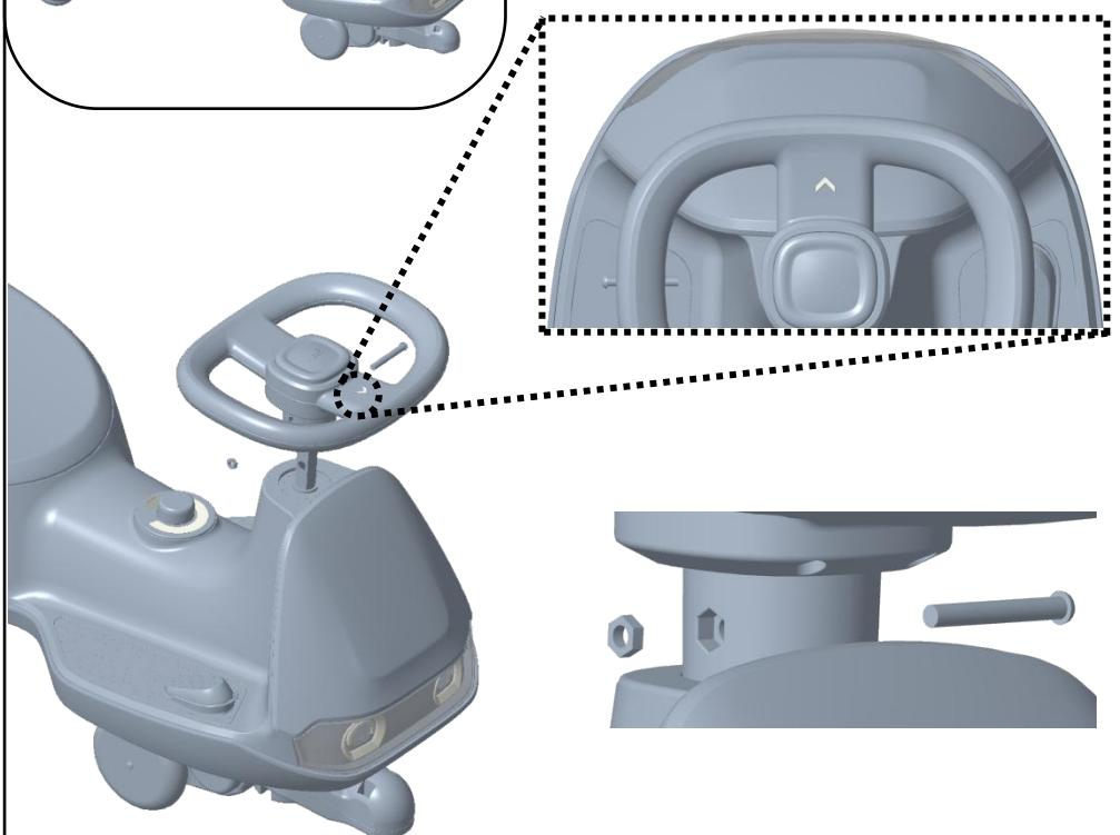
Insert the steering wheel into the square tube in the direction shown in the diagram (with the steering wheel arrow pointing toward the front of the vehicle). Use the included M5 bolt and nut to secure the steering wheel to the square tube (please place the M5 nut in the corresponding hexagonal groove).
