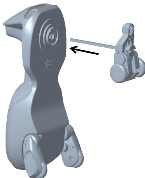
Pass the square tube that has been fixed to the Drive device through the circular hole in the bottom of the vehicle, and rotate the Drive device until it aligns with the direction shown in the diagram.
