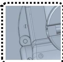
The vehicle is set to high speed by default at the factory. You can use a tool to reach into the circular hole in the bottom of the vehicle and adjust the internal switch to the low-speed gear.
