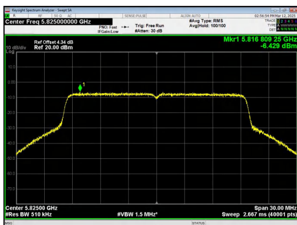
(802.11ax20) PSD plot on channel 165
