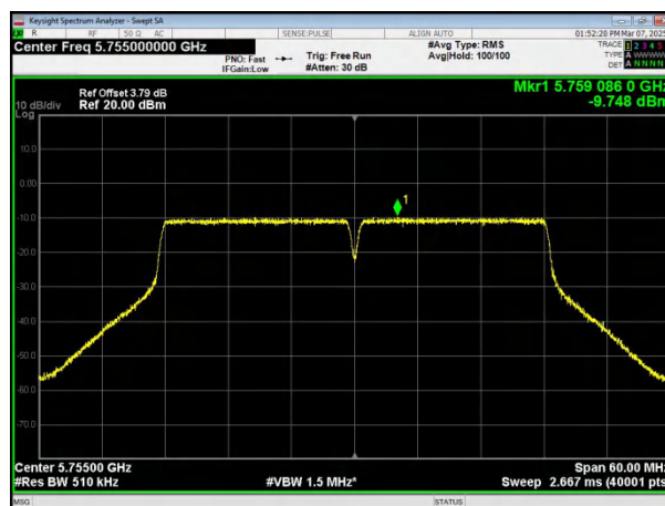
(802.11ac40) PSD plot on channel 151
