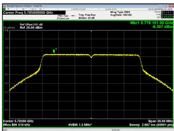
(802.11ac20) PSD plot on channel 157
