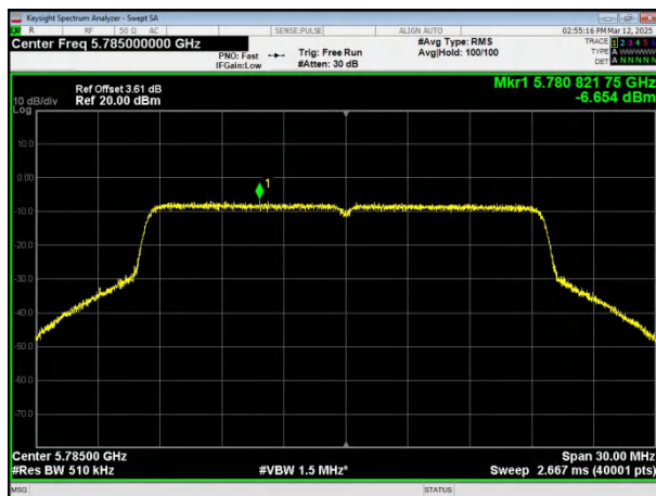
(802.11ax20) PSD plot on channel 157
