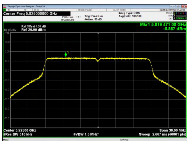
(802.11ac20) PSD plot on channel 165
