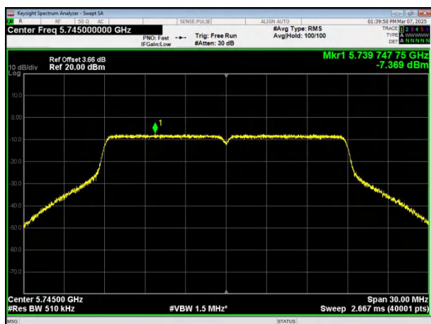
(802.11ac20) PSD plot on channel 149
