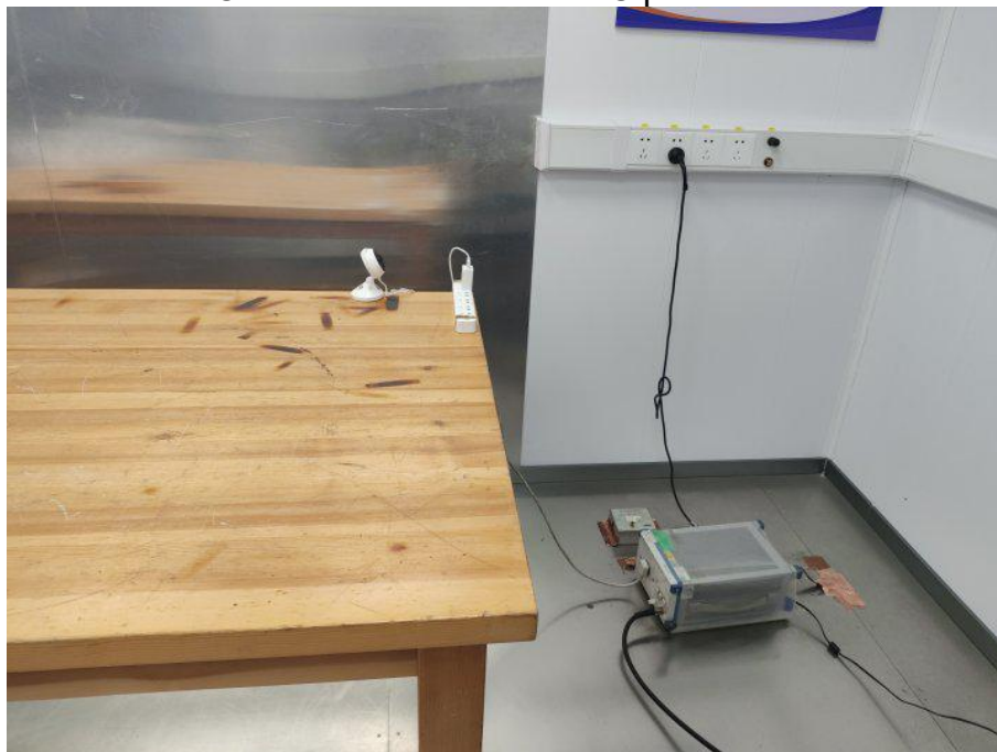
Conducted Emission at AC power line
