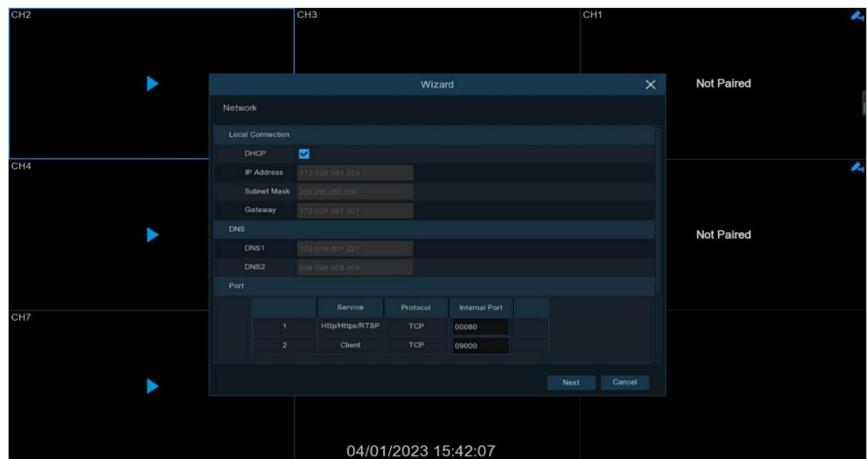
If the network to which the device is connected has a DHCP server, you can check the DHCP box, and the DHCP server will automatically assign all network parameters to the device. Alternatively, you can manually set the IP
