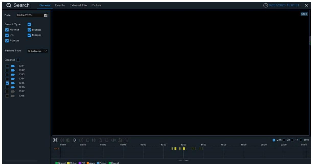
In the playback interface, users can perform operations such as play/stop/single frame playback/clipping/backup, etc. The NVR also supports playback modes such as time slicing, events, and images. Please refer to the user manual for more information.
