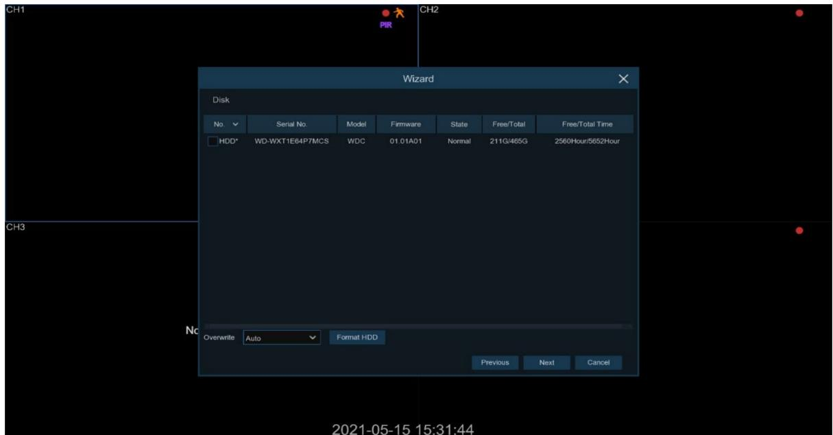
When the hard disk is first installed on the NVR, it needs to be formatted. Select the hard disk and then click the "FormatHDD" icon to format the hard disk.
