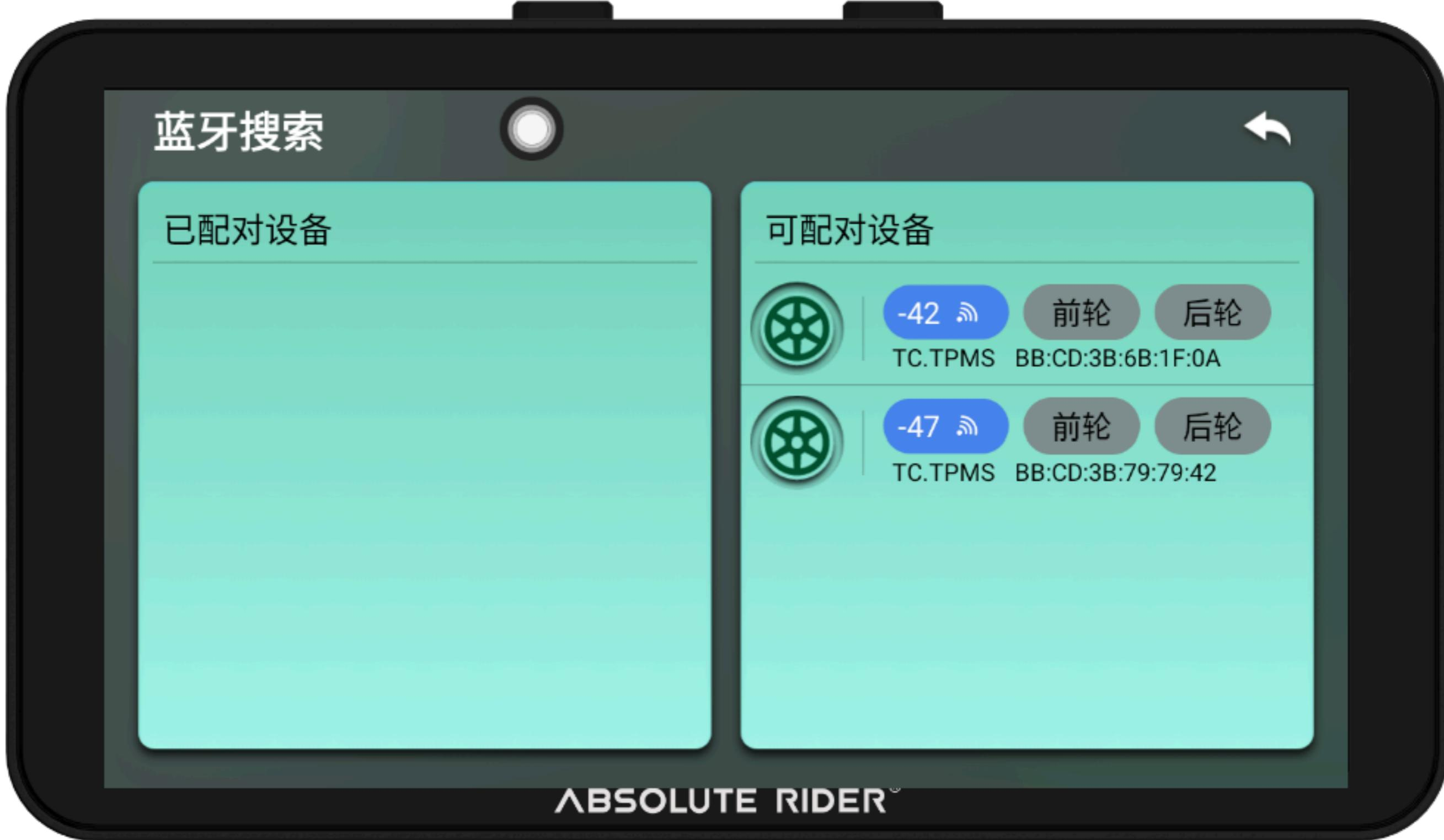
3 When the main unit starts to search for signals, the external module installed on the corresponding tire will send its ID information for pairing selection.
