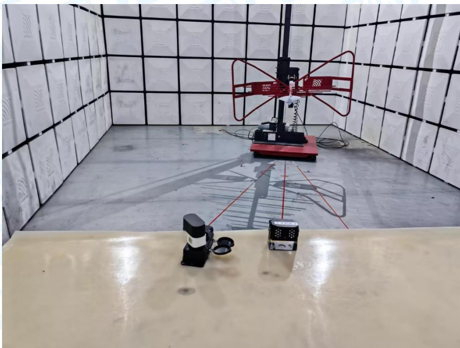
Photo of Setup for Radiated Emission (30MHz~1GHz)
