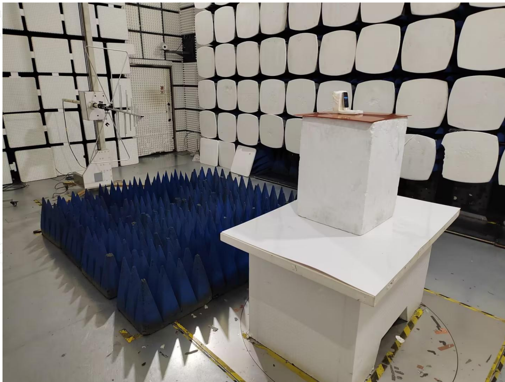
Radiated Emissions Measurement (Below 1GHz)
