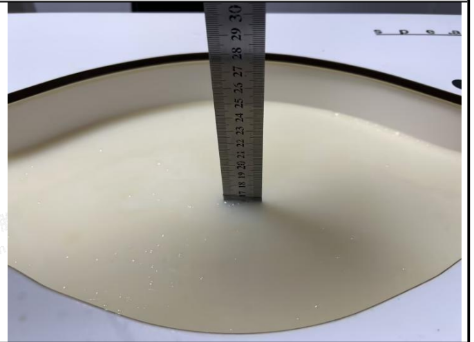
Photo 2: Tissue Simulant Liquid for Head 3000-8000MHz
