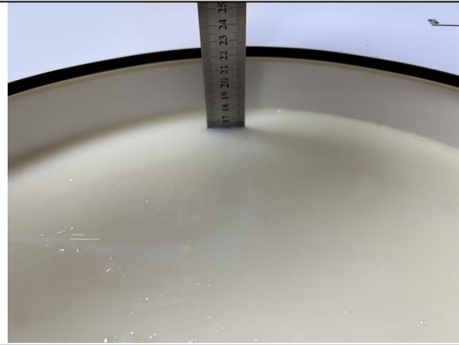
Photo 1: Tissue Simulant Liquid for Head 700-3000MHz
