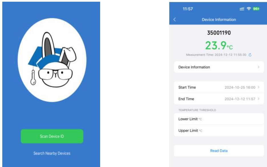
3、The app interface shows the device's current temperature data and time. Also, it allows checking device info, set the time range for viewing the collected data, temperature threshold range, and reading monitoring data.
