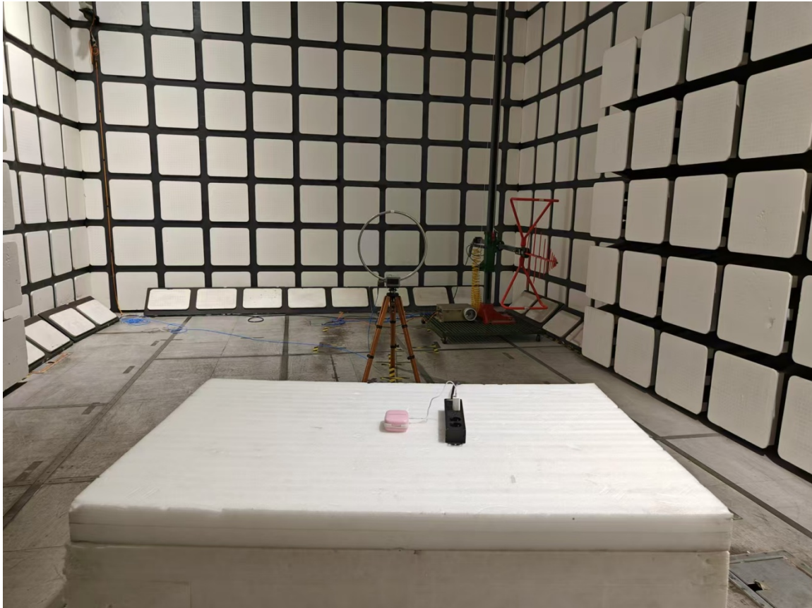
Radiated Emissions View (Below 1 GHz)
