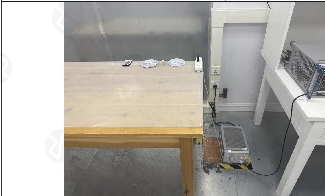
Conducted Emission at AC power line
