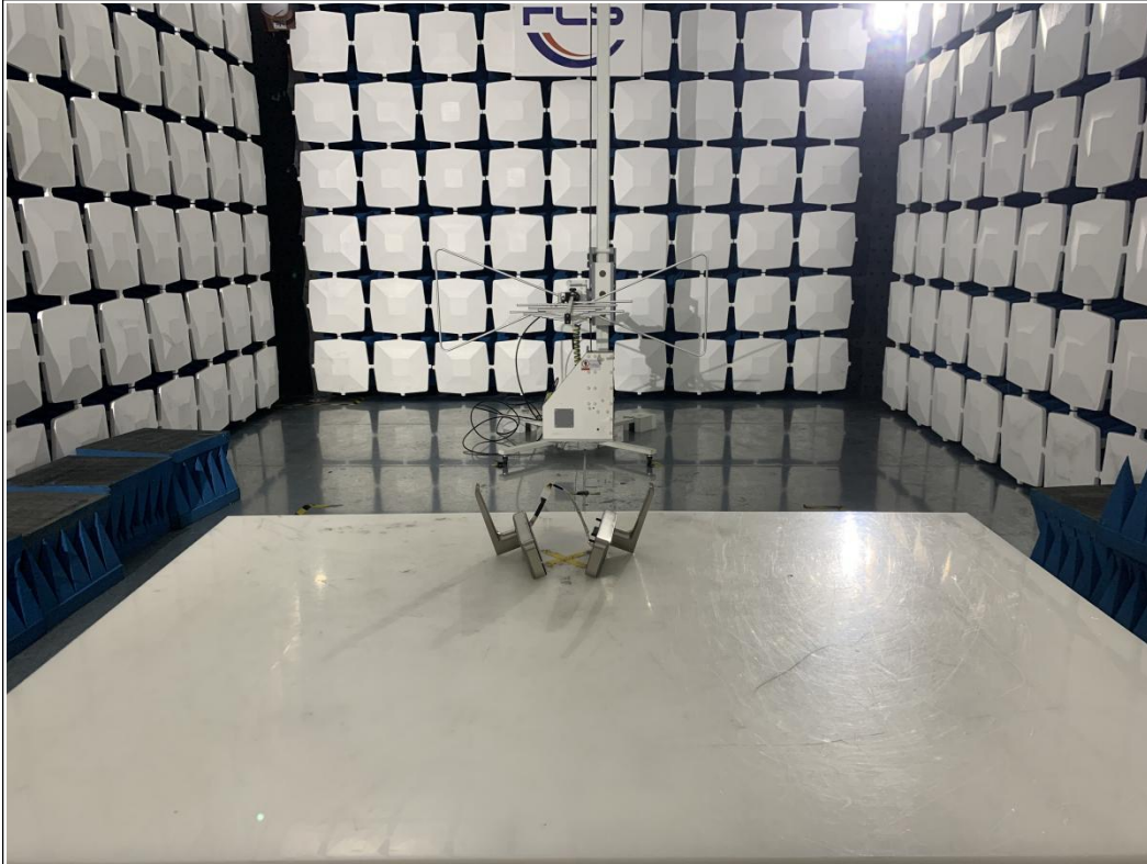
Above 1GHz for radiated emission test setup
