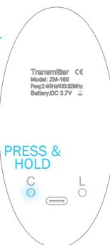
**2** Check the direction of the motor by pressing **▲** or **▼** and ensure that it is moving in accordance with the remote control. To change the direction, press and hold the **L** and **■** buttons until the motor jogs once.
