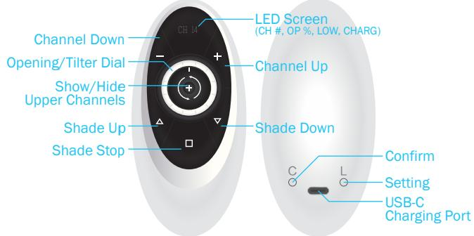
**1** Switch motor **ON**, press and hold **SETTING** button until you see the motor jog once – motor will now be in pairing mode. On the remote control, select a channel by using - or + button. On the back of the remote, press and hold **C** button until motor jogs once.
