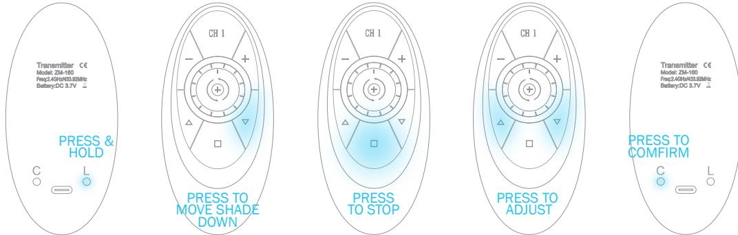
**4** To set upper limit, press **▲** button to move shade up to desired top position and then press **■** to stop shade. To adjust, press **▲** or **▼** according to your needs. Press **C** button to confirm and motor will jog twice.
