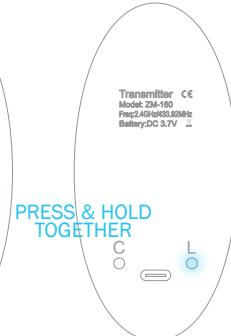
**3** To set limits, press and hold **L** button until you see motor jogging once. To set bottom limit first, press **▼** button to move shade down to desired bottom position and then press **■** to stop shade. To adjust, press **▲** or **▼** according to your needs. Press **C** button to confirm and motor will jog once.
