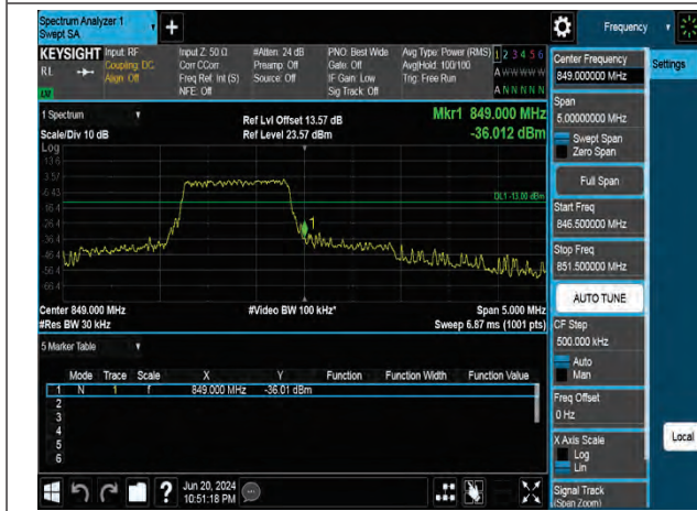
QPSK High channel-6 RB offset 0
