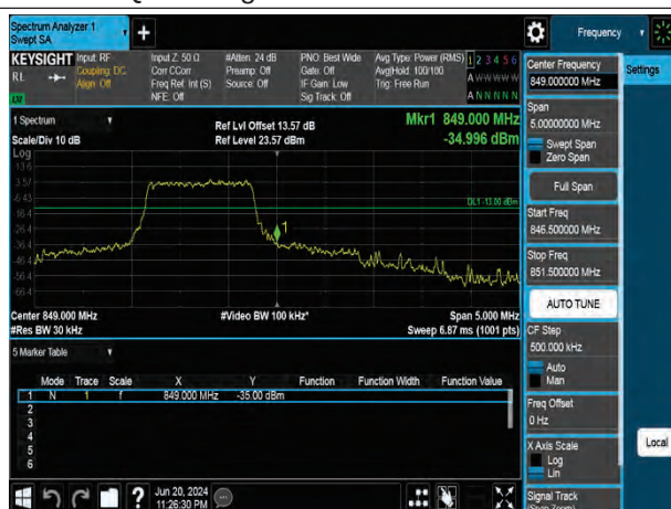
QPSK High channel-6 RB offset 0
