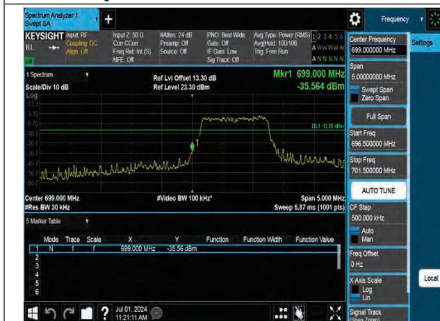
QPSK Low channel-6 RB offset 0
