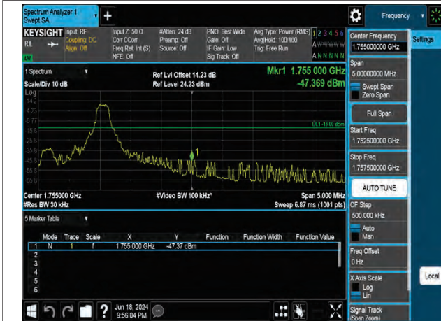
QPSK High channel-6 RB offset 0
