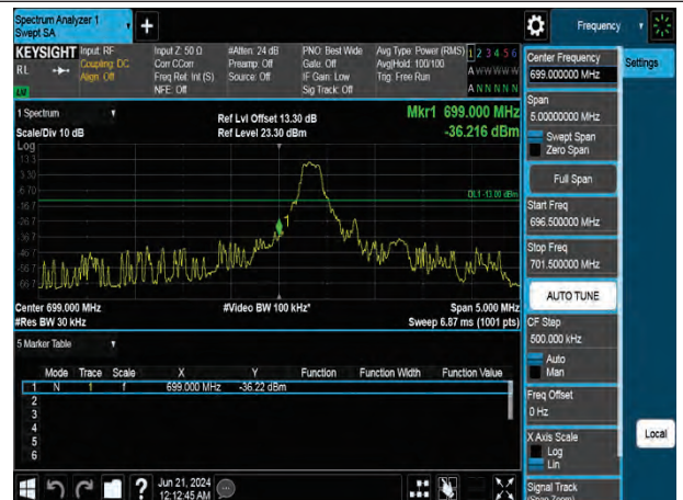
16QAM Low channel-1 RB offset 0
