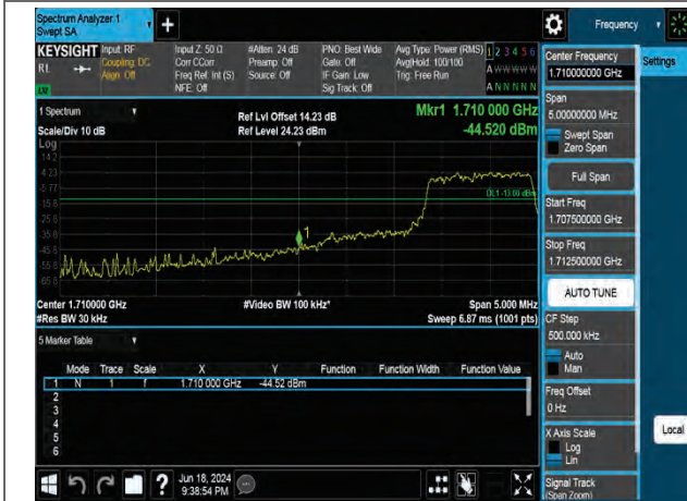
QPSK High channel-1 RB offset max
