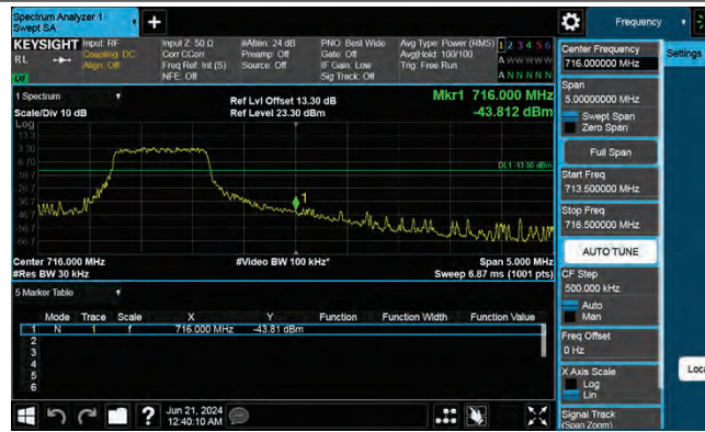
16QAM High channel-5 RB offset 0
