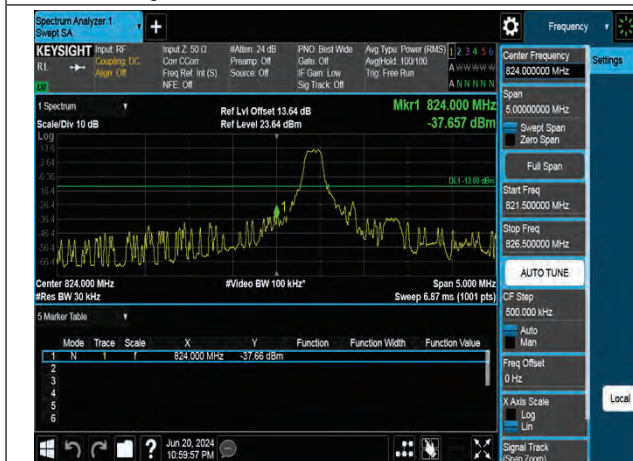
QPSK Low channel-6 RB offset 0
