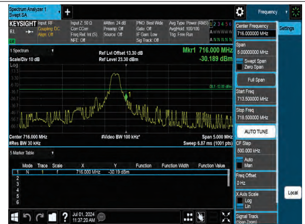
16QAM High channel-5 RB offset 0
