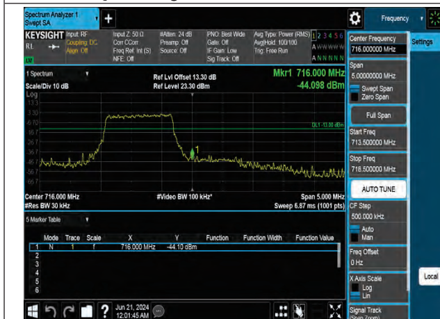
QPSK High channel-6 RB offset 0
