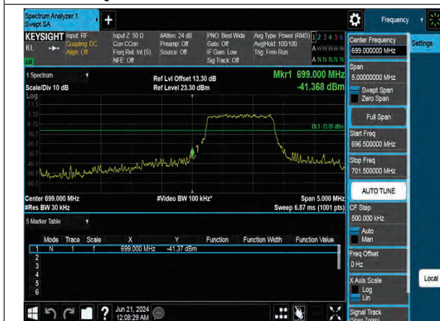
QPSK High channel-1 RB offset max
