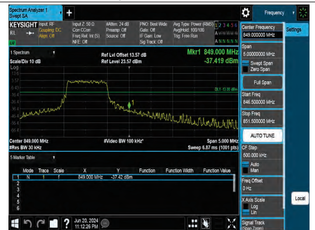
16QAM High channel-5 RB offset 0
