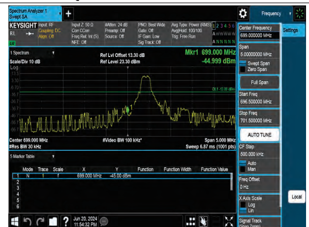
16QAM Low channel-1 RB offset 0
