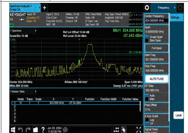
16QAM Low channel-5 RB offset 0
