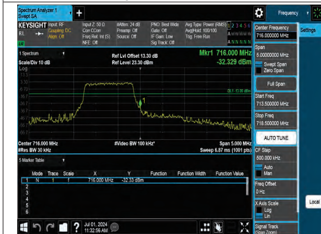
QPSK High channel-6 RB offset 0
