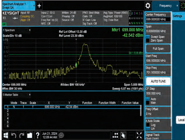
QPSK Low channel-1 RB offset 0
