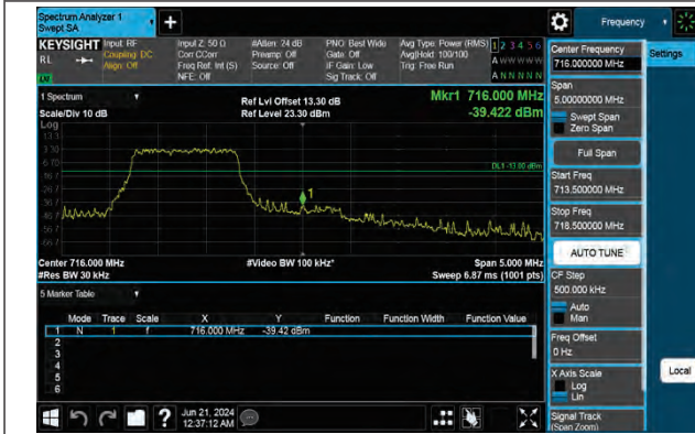
QPSK High channel-6 RB offset 0
