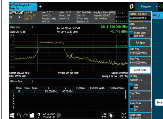
QPSK High channel-6 RB offset 0
