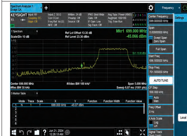
QPSK Low channel-6 RB offset 0
