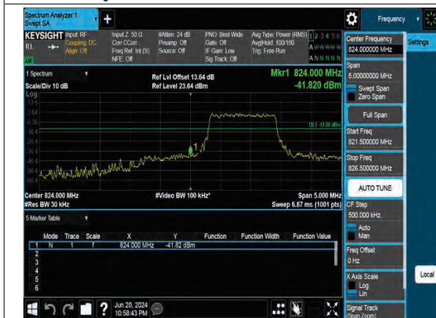
QPSK Low channel-6 RB offset 0
