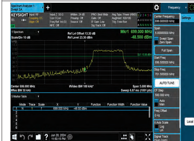
QPSK High channel-1 RB offset max
