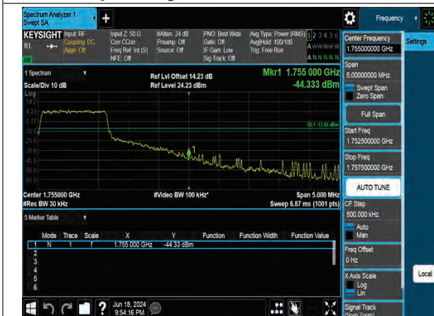
QPSK High channel-6 RB offset 0
