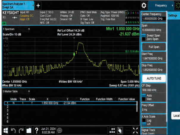
QPSK Low channel-1 RB offset 0
