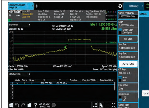
QPSK High channel-1 RB offset max
