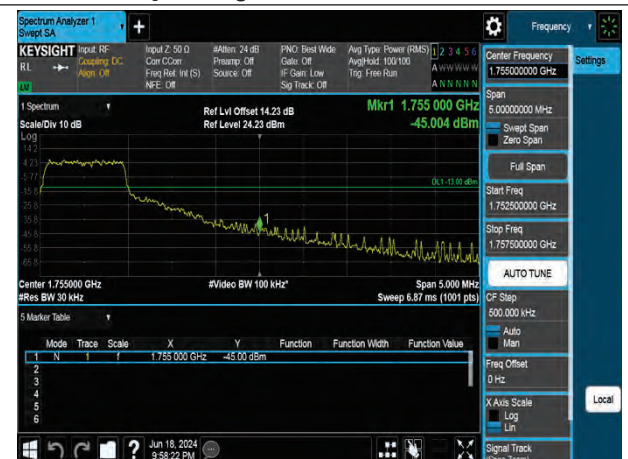
16QAM High channel-5 RB offset 0
