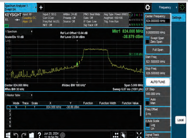
16QAM Low channel-5 RB offset 0
