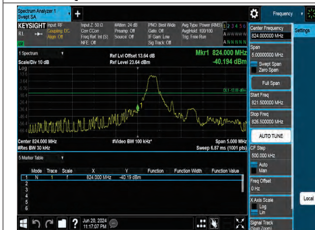
QPSK Low channel-1 RB offset 0
