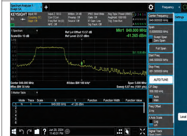
QPSK High channel-6 RB offset 0
