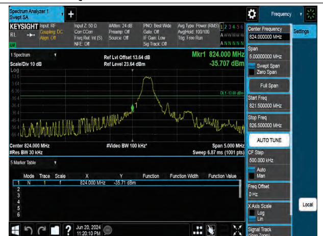
16QAM Low channel-1 RB offset 0
