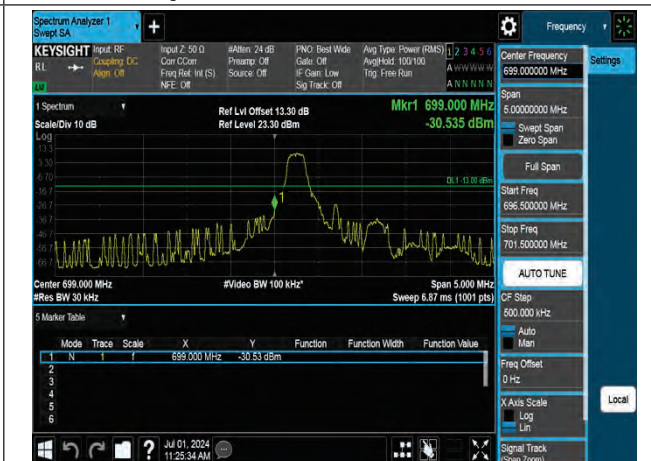
16QAM Low channel-5 RB offset 0
