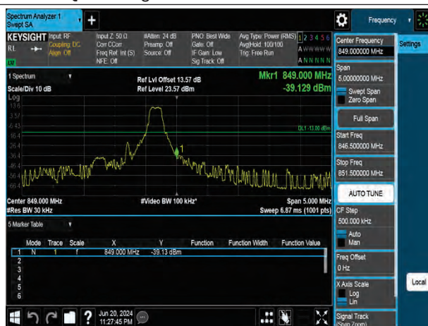
QPSK High channel-6 RB offset 0
