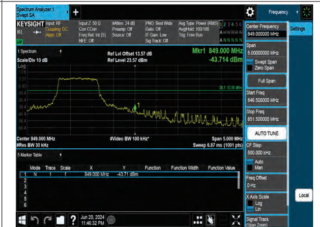
16QAM High channel-5 RB offset 0
