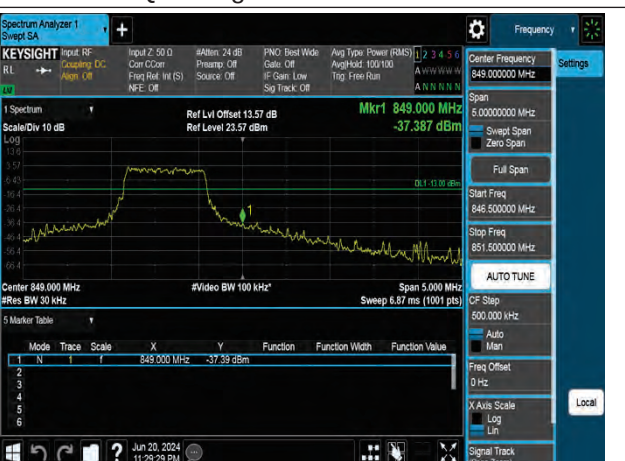
16QAM High channel-6 RB offset 0
