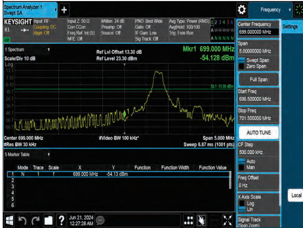
QPSK Low channel-1 RB offset 0
