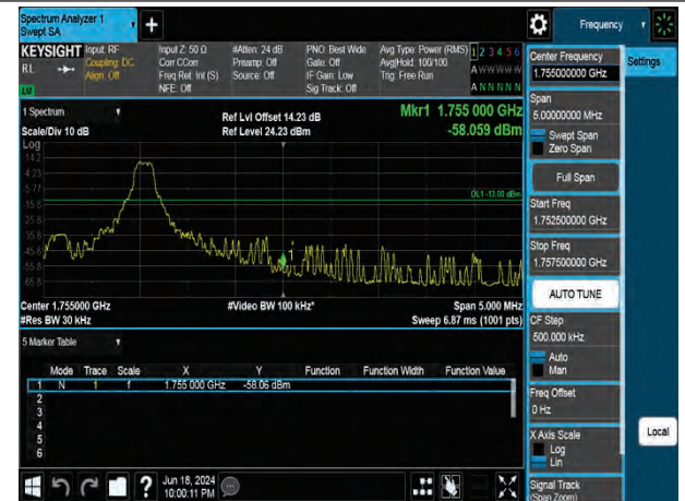
16QAM High channel-5 RB offset 0
