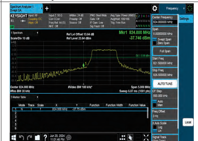
16QAM Low channel-5 RB offset 0
