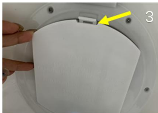
Figure 2-12 Battery replacement: Ejection (left 3 figures) and Insertion (right 3 figures)
