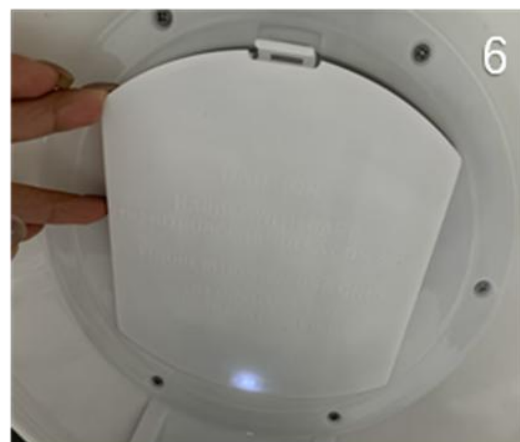
Figure 2-12 Battery replacement: Ejection (left 3 figures) and Insertion (right 3 figures)
