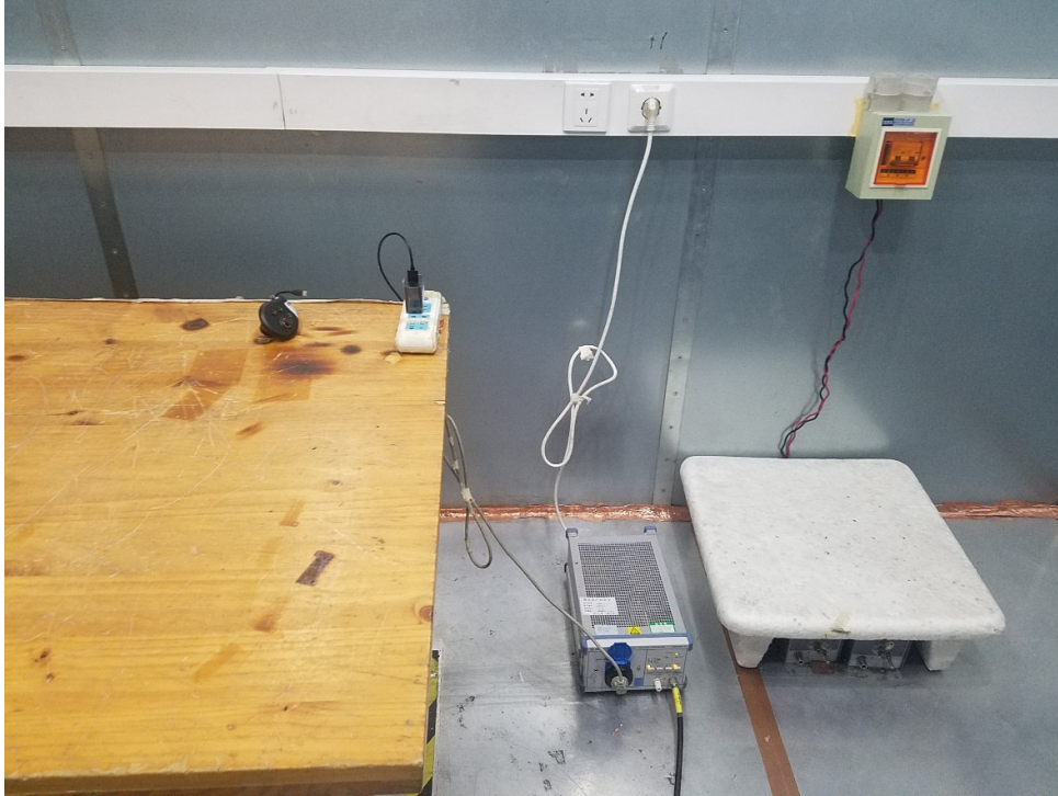
Picture 2: Conducted Emissions Test Setup
