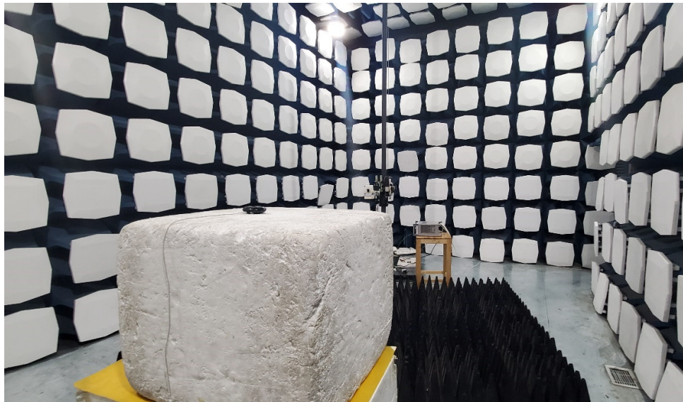
Picture 1 Radiated Emission Test Setup
