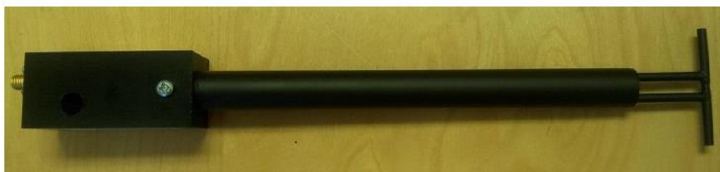
Figure 1 – MVG COMOSAR Validation Dipole
