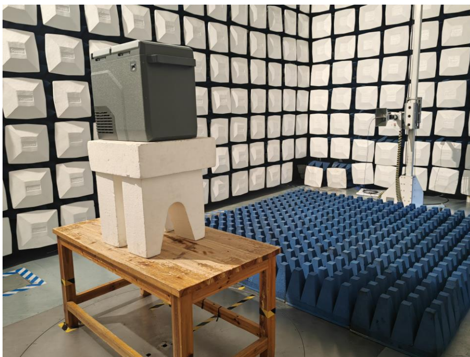
Test Setup For Radiated Emission (Above 1GHz)
