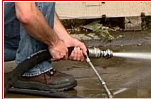
**Fig 11. UHP Tube Flushing**
