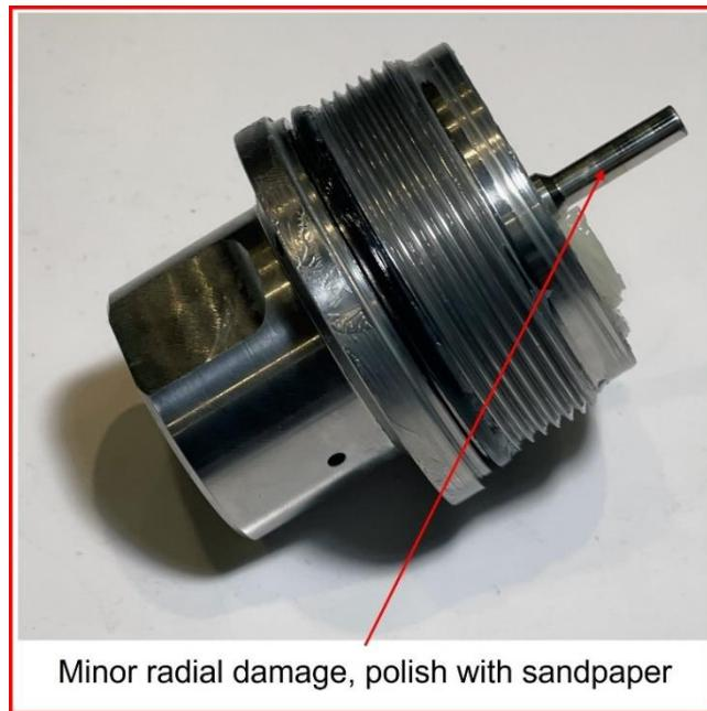
**Fig 17. Sealing Rod Maintenance**
