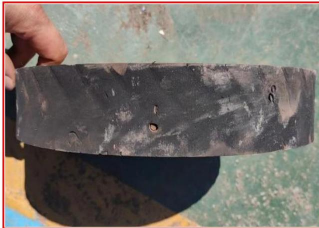
**Fig 28. Driving Wheel Needs to be Replaced**
