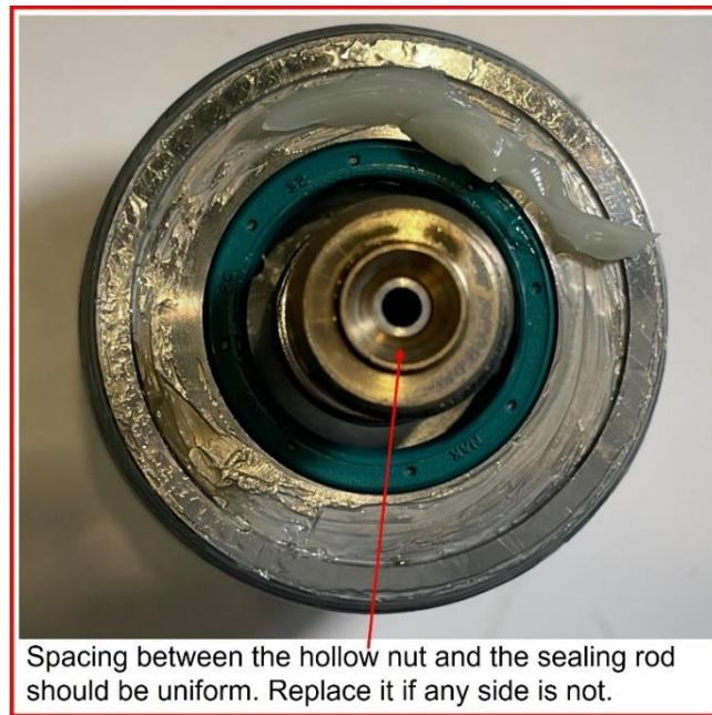
**Fig 19. Hollow Nut Maintenance**
