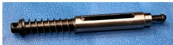
**Fig 20. HP Seal Disassemble Tool**
