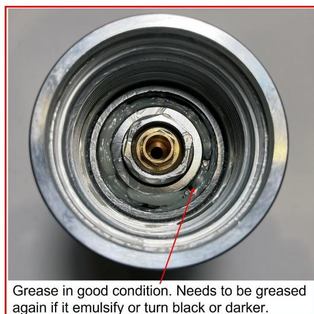
**Fig 16. Greasing the Rotary**
