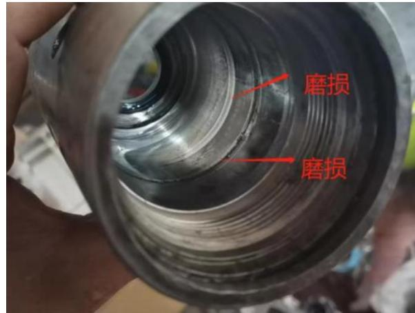
**Fig 22. Worn Rotary Shell**
