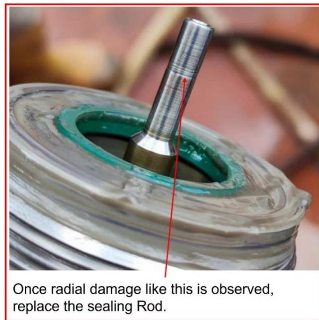
**Fig 18. Sealing Rods Needs to be Replaced**
