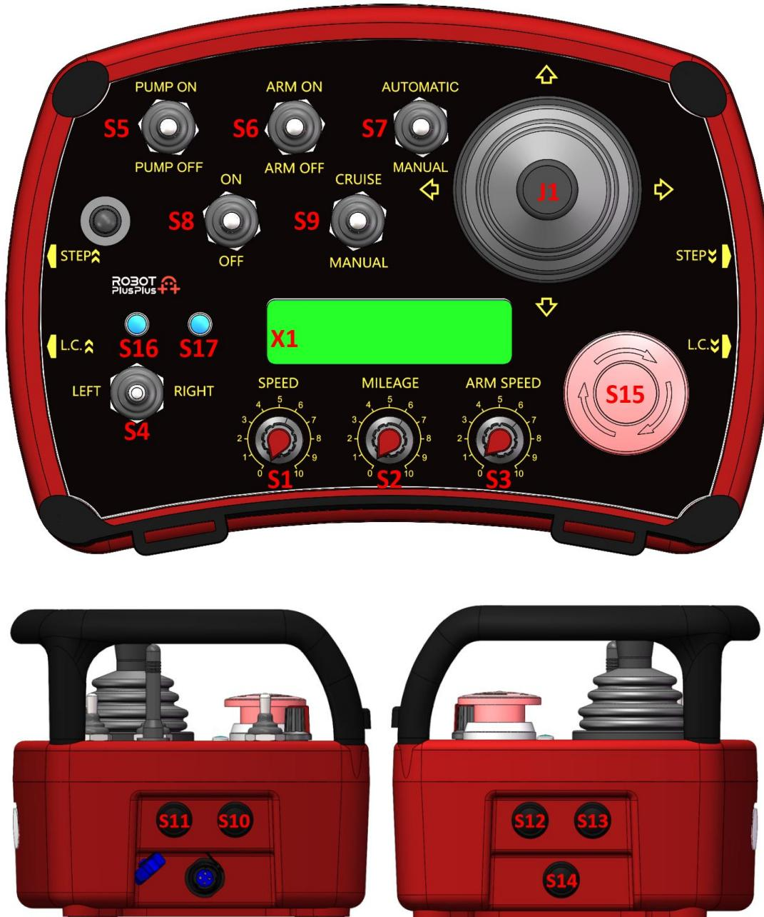
**Fig 5. Different Views of the Remote Control**
