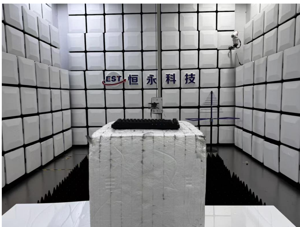
Radiated emission test: Above 1GHz
