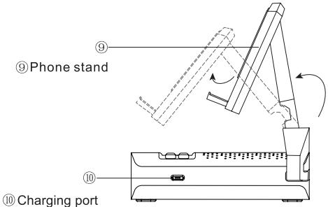
When the phone stand is folded, this lever is locked. Please pull up this lever first, then you can adjust the height of the phone stand.
