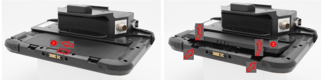
Figure 3-1 Remove the battery
