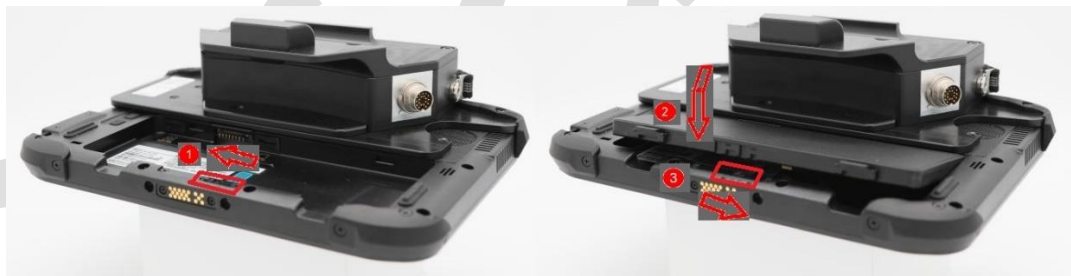
Figure 3-2 Insert the battery
