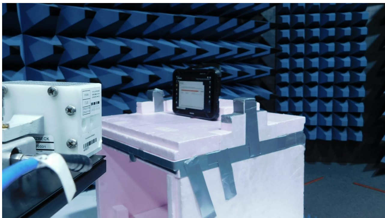
Picture 7: FS-SAC, radiated emission test 17 GHz – 26 GHz (front view)
