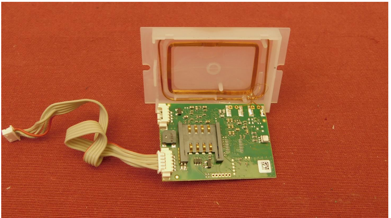
Picture 6 PCB of RFID module bottom side
