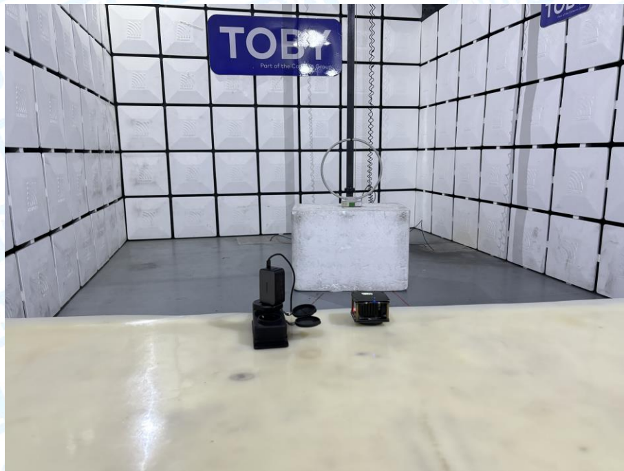
Photo of Setup for Radiated Emission (9KHz-30MHz)
