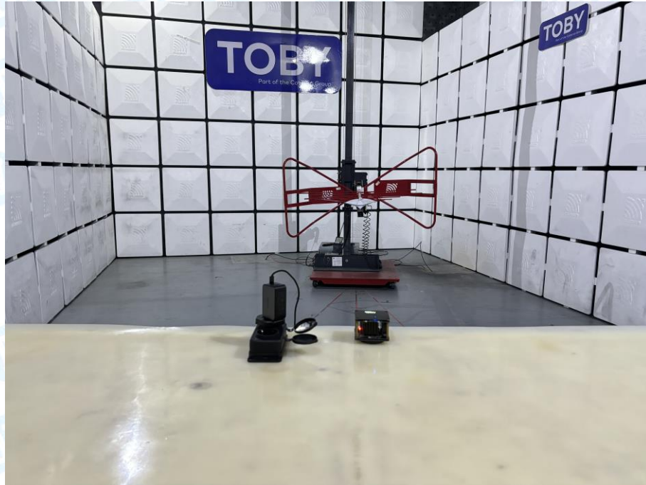
Photo of Setup for Radiated Emission (9KHz-30MHz)
