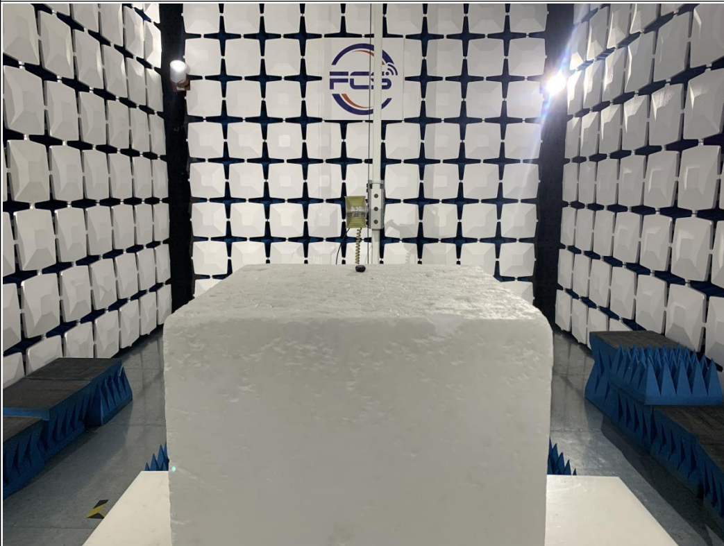
Above 1GHz for radiated emission test setup
