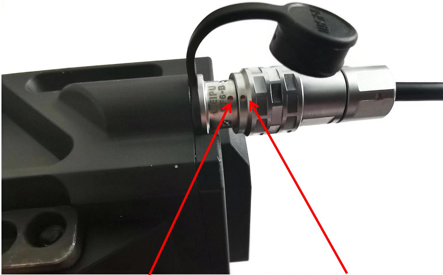
Install the aviation plug in the direction indicated by the plug as shown in the picture. Please find the **correct direction** of the pins and the holes !!!
