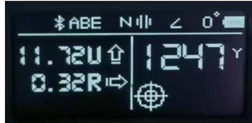
ABI means AB Inside mode, and it has the AB apps inside and after the device measure the distance, it would calculating the ballistic figure in order to show to you the complete solution.
