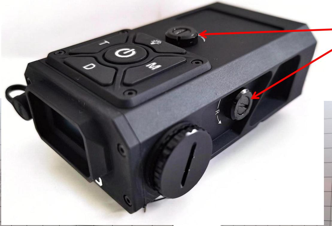
By adjusting the up and down , left and right adjustment wheels of the ballistic computer, the position of the red visible laser is changed to make it coincide with the highly reflective circular target paper
