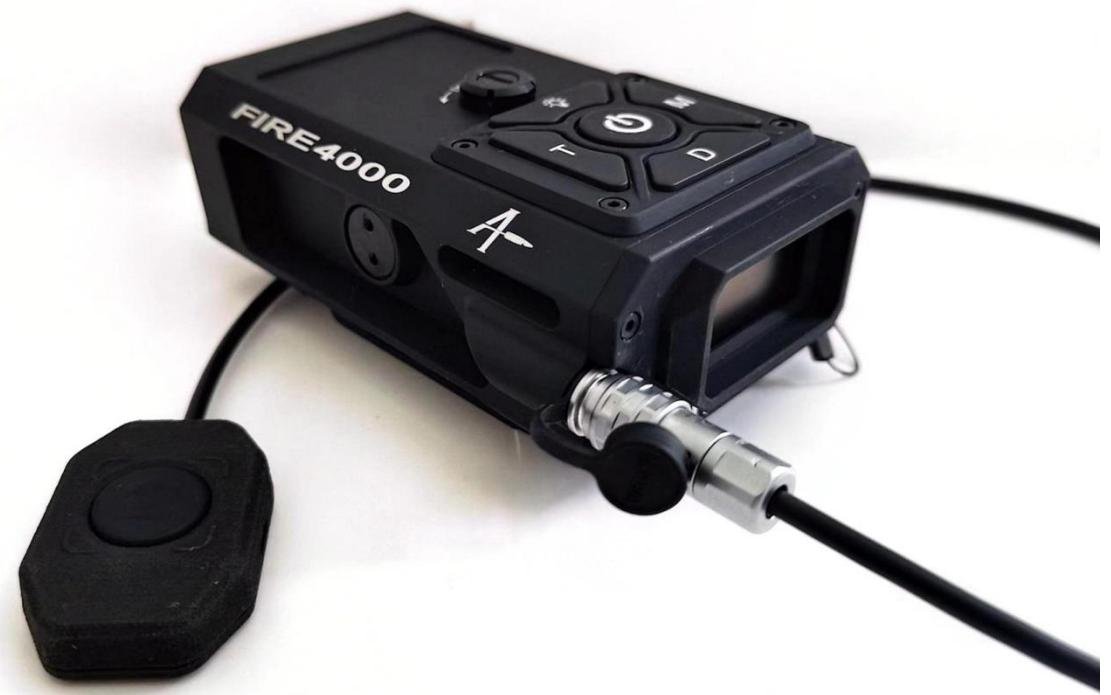
Install the aviation plug in the direction indicated by the plug as shown in the picture ! ! !
