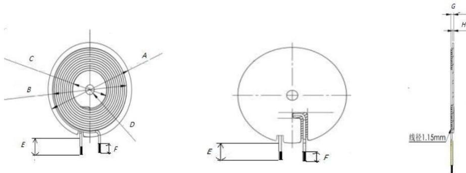
Remark: Coil lead-out position winding 5MM ( ref ) High temperature adhesive , the back of magnetic sheet with double-sidedgum.
