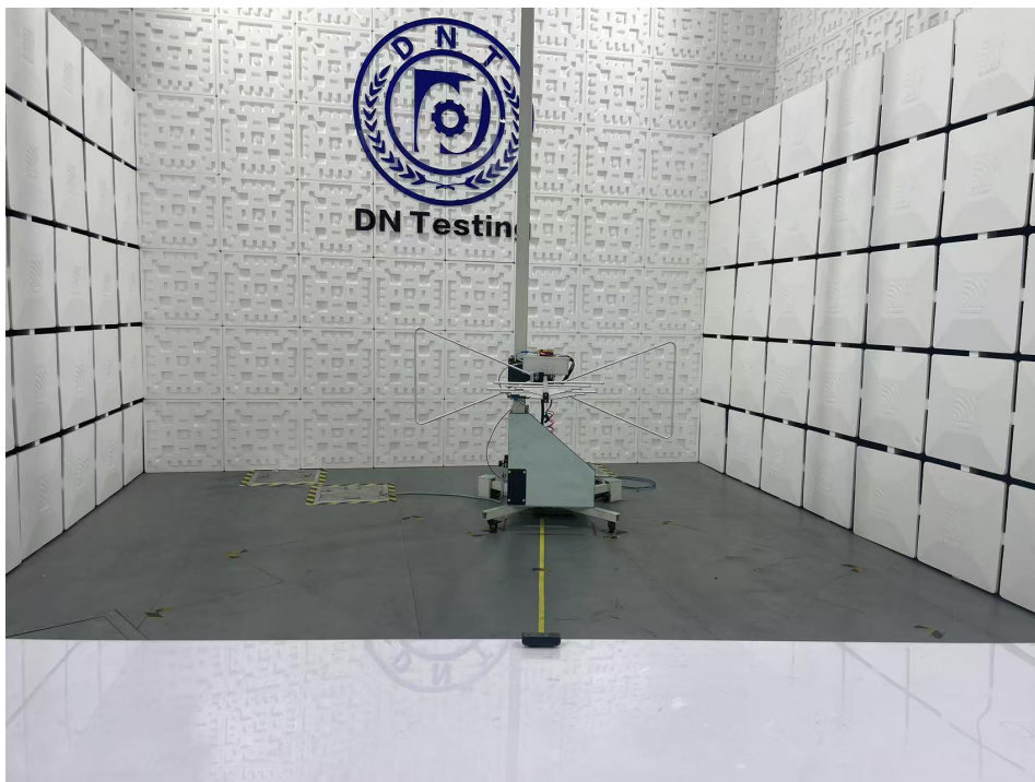
Radiated Emission Test View|(Below 1G)
